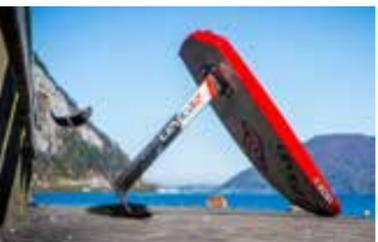
>> Hydrofoil board: when adequate speed = lift is reached, the board rises out of the water.
