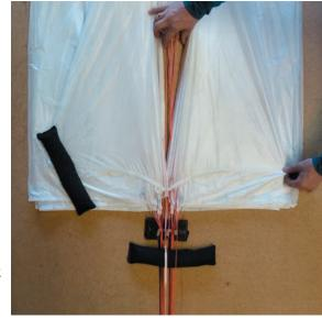
10. The extra material simply can be pushed up inside the channel as in the picture.The reason for this is to prevent the material from burning during a deployment.
