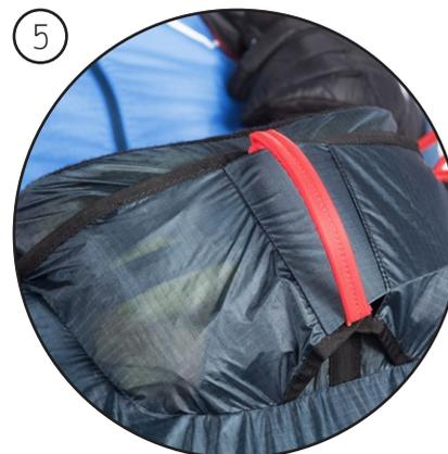
The front reserve chute system is located on the upper side of the pod and doubles as a cockpit thanks to its convenient position.
