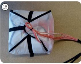
16. Starting at the main riser, loop the line bundles in the shape of a figure-eight. Use silicone-based rubber rings to fix the line bundles.Make sure that there is no line knot in the line loop. Make sure to leave approx. 30 cm free to the first figure-eight. This length is needed for the
