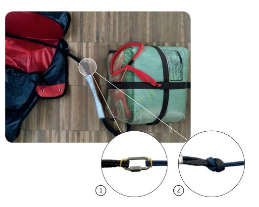
It is important to ensure that the connection is centered, that is, the two connecting lines leading to the shoulder straps are of the same length. If the harness does not have an integrated attachment possibility for the reserve chute on the shoulder straps, then the reserve chute connecting line can also be attached to both main carabiners.
