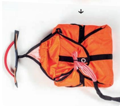
4. Now you can connect the V-lines of the BREEZE with the lanyard of your reserve chute. To connect the reserve chute to the V-line, you must use a screw shackle with at least 2400 daN strength. The lines have to be connected on both sides of the screw shackle and must be secured with rubber bands (pic 1).
