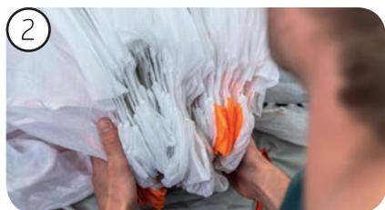
2 Lay the Rigid Foils of the leading edge on top of one another. It's best to start from the middle and work on one half of the glider, then do the second half and place its Rigid Foils next to those of the first half.
