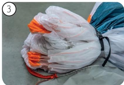
3 Turn the entire leading edge 90° on its side and fix the glider with the first compression band to the Softbag.
