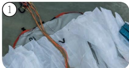
1 Gather up your glider and place it on the Softbag. At the bottom of the Softbag is a toggle button where you can attach the risers later. The trailing edge of the glider should lie in the direction of the toggle button.
