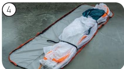
4 Now sort the rest of the glider lengthwise to the trailing edge and fix it with the remaining compression bands.
