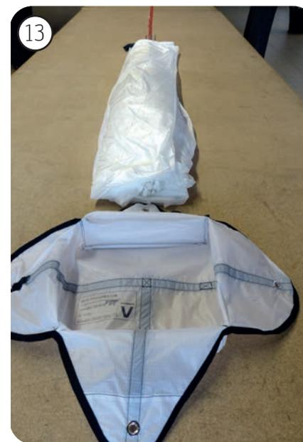
13. Now fold the reserve chute with a "double S-fold" or use the "simple S-fold" for sizes 180 & 225 and place the reserve container with the line pocket in the direction of the base/main riser.
