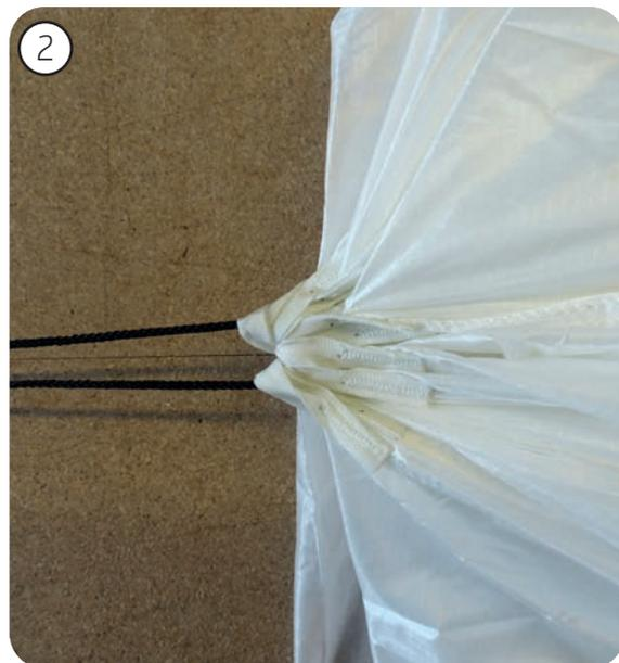
2. Secure the packing loops for now and pull on the main riser and the attached loops until it is tight.
