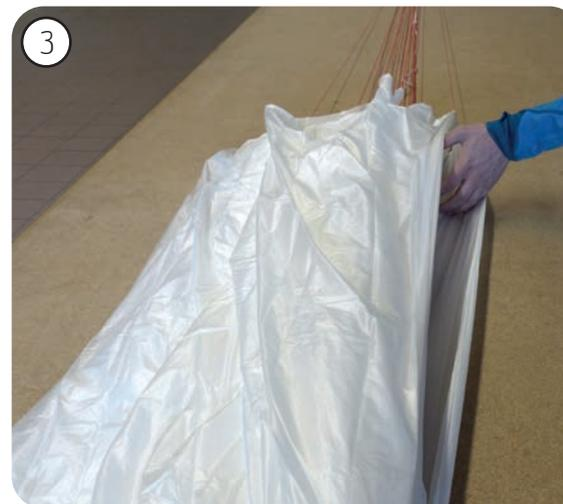
3. The PEPPER CROSS LIGHT is a cruciform rescue parachute with four corner points, so lay out the canopy with one corner at the bottom, one on the left, one on the right and one on top. Start with the first corner at the bottom and smooth the material by running your hand along it on the table.
