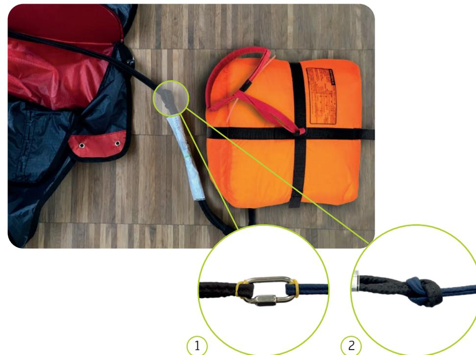
It is important to ensure that the connection is centered, both connecting lines that lead to the shoulder are of the same length. If the harness does not have an integrated attachment possibility for the reserve chute on the shoulder straps, then the reserve chute connecting line can also be attached to both main carabiners. For removal proceed in reverse order.
