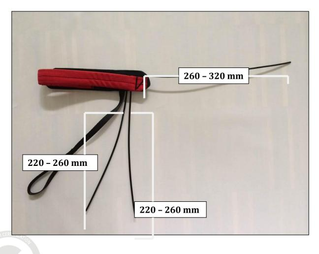
If the actual length is shorter than the indicated values, the container can be inadvertently open and cause the rescue equipment to fall out. In the worst case it can fall out during flight without the pilot noticing.
