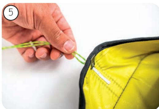
6. First close the lower flap with the numbering 1-3 and attach the loop with the pin of the rescue grip. Make sure that the rescue grip is mounted the right way round, otherwise the connecting strap will cover the velcro. Remove the piece of line on this side.
