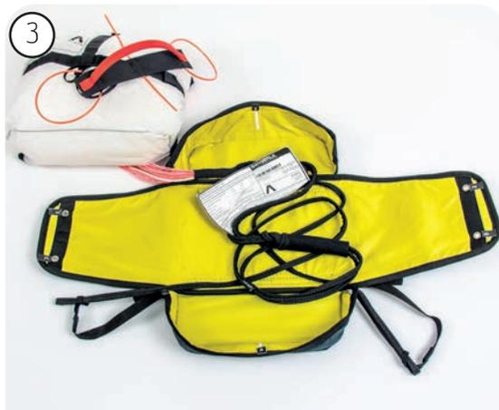
4. Guide the V-line to the left and right of the cover flap (with velcro on top) and make sure that you have enough V-line from the front container depending on the type of assembly (main carabiner or shoulder harness mount).
