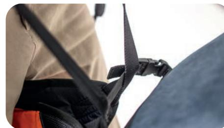
All three attachment points offer the possibility to adjust the length of the attachment. Make sure that the fasteners are neither loose in flight nor take the main tension of the harness.
