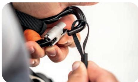
When using this method make sure that the speed bar connecting line is always routed between the harness and the V-line.
