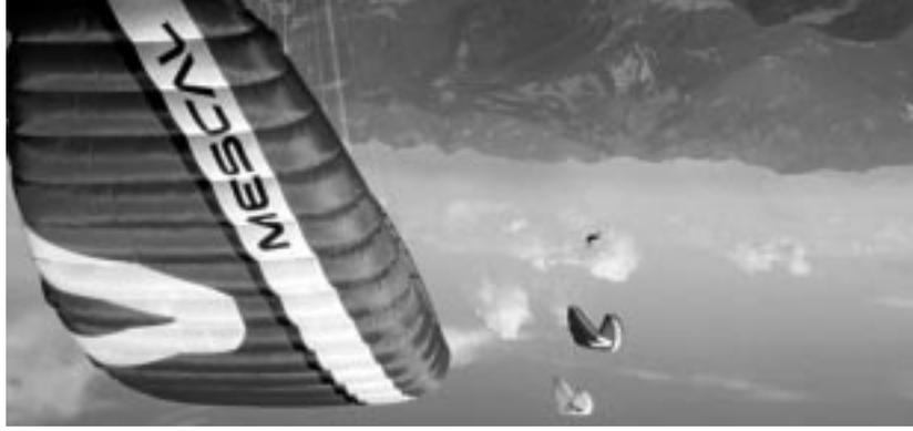
**AS SOON AS YOU APPLY THE BRAKES DURING A PARACHUTAL STALL THE PARAGLIDER WILL IMMEDIATELY ENTER A FULL STALL. IF STILL IN A PARACHUTAL STALL CLOSE TO THE GROUND DO NOT ATTEMPT TO RECOVER BUT STRAIGHTEN UP YOUR POSITION IN THE HARNESS AND PREPARE FOR A PARACHUTE LANDING ROLL.**
