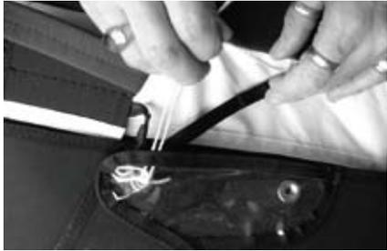
5. Insert the pack laces into the loops. First pull the helpline on one side through the grommets of the lashes one after the other. Stick the splint through the loop.
