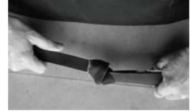
2. Secure with an elastic to ensure against slippage. As an alternative you can use a steel shackle.
