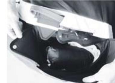
4. Insert Rescue Handle in the loop fastener of the inner container and place into the outer container as illustrated. Be careful that the connection between the loop fastener and Rescue Handle end in an upwards facing position (to the protector). Otherwise, by deployment there is a danger of jamming.
