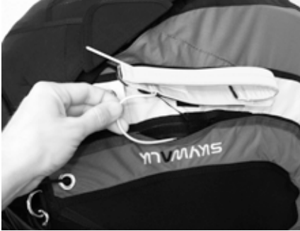
13. Insert unused Splint A backwards in the channel of the Rescue Connection
