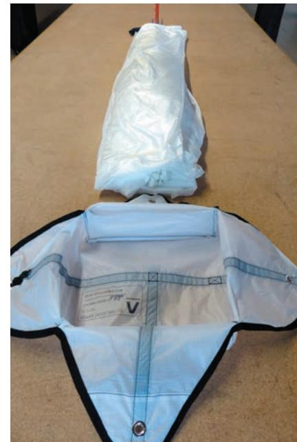
13. Now fold the reserve chute with an „S-fold“ corresponding to your size and place the rescue container that the rescue flap with the rubber loop looks to the side (seen from the base).
