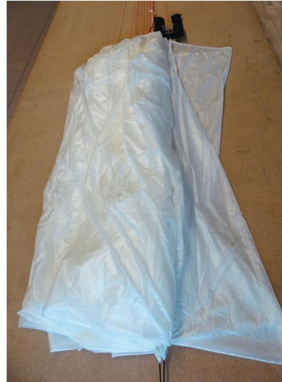
4. Pull the base from one line attachment point to the next along the seam to the side you are sorting and smooth the crossed panel. A line separator and a weight will help to secure the already sorted lines.
