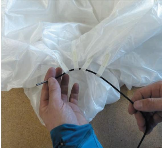
2. Secure the packing loops for now and pull on the main riser and the attached loops until it is tight.
