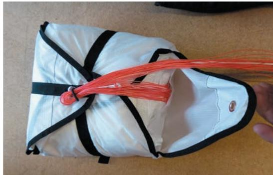
**16.** Starting at the main riser, loop the line bundles in the shape of a figure-eight. Use siliconebased rubber rings to fix the line bundles. Make sure that there is no line knot in the line loop. Make sure to leave approx. 30 cm free to the first figure-eight. This length is needed for the final line loop.
