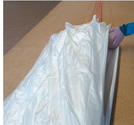
3. The TAPA X-ALPS is a cruciform rescue parachute with four corner points, so lay out the canopy with one corner at the bottom, one on the left, one on the right and one on top. Start with the first corner at the bottom and smooth the material by running your hand along it on the table.
