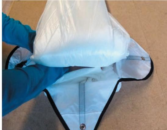
**15.** Now close the first three rescue flaps and secure them with a small line loop. This method will avoid burns from a deployment later since the bundle of lines will be released first and will not come in contact with the material.
