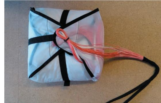
**17.** Place the line bundles in the fourth and final rescue flap and secure it with the remaining line length from step 16.
