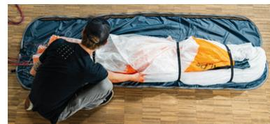
Now sort the rest of the canopy lengthwise to the trailing edge, making sure that the Rigid Foils lie neatly lengthwise and are not twisted.
