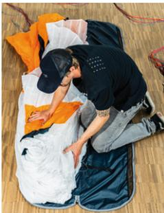
With this technique, the glider lies together like an accordion from wing tip to wing tip and is not folded in the center of the glider. Thus, neither the center cells nor the Rigid Foils are subjected to increased stress. The openings at the leading edge must be aligned with the center of the Softbag.
