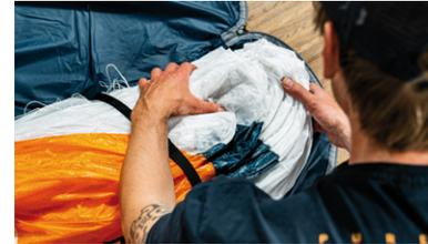
Make sure that the openings at the leading edge are neatly aligned. The Rigid Foils on the stabilos must also be pulled up towards the remaining leading edge.
