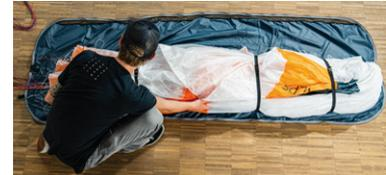
Now sort the rest of the canopy lengthwise to the trailing edge, making sure that the Rigid Foils lie neatly lengthwise and are not twisted.
