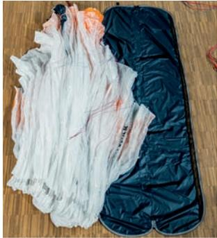
Gather your glider and lay it next to the Guardbag. The lines should protrude out of the trailing edge. At the bottom of the Guardbag there is a riser bag, here the risers will be stowed away later. The trailing edge should be in the direction of the riser bag.
