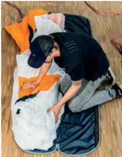
With this technique, the glider lies together like an accordion from wing tip to wing tip and is not folded in the center of the glider. Thus, neither the center cells nor the Rigid Foils are subjected to increased stress. The openings at the leading edge must be aligned with the center of the Guardbag.
