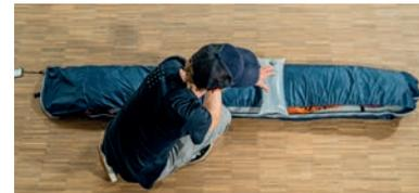
Carefully close the zipper, being careful not to pinch any lines or paraglider material. Place the packing tube at the level of the second webbing strap.
