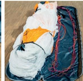
Stow the risers into the riser bag and place the lines into the Guardbag.
