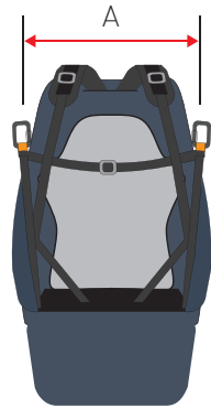
Width of harness attachment points
