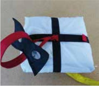
When installing the rescue parachute in the RANGE AIR front container, be sure to attach the rescue handle to the loop in the middle of the rescue parachute and not to a loop on the side. Connect the rescue parachute to the V-bridle using a shackle with at least 2400 daN mechanical strength, such as a Maillon Rapide 6mm screw shackle.
