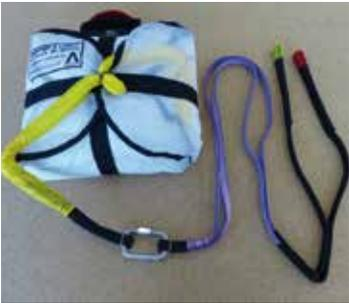
Secure the connecting lines on both sides of the shackle with rubber rings. The use of webbed straps is not recommended because they can slip if the attachment is asymmetric and could tear due to the high heat of friction during a rescue deployment.
