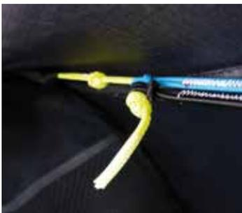
On the front of the seat you will find additional attachment loops on each side that should also be used to attach the line to the desired position on the bottom of the footboard using the same knot.
