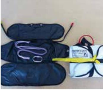
Lay the front container in front of you as in the photo below and place the lines of the V-bridle in a S-shape neatly and without twisting in the container. Make sure that both ends of the V-bridle (red for the left side, green for the right side) stick out of the container toward the velcro cockpit and are connected to the inside of the velcro.
