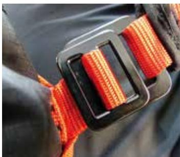
Before every launch, close the “get up” system with the two frame buckles and connect the reserve parachute to the harness by hooking the ends of the two V-bridle lines into the main carabiner on each side.
