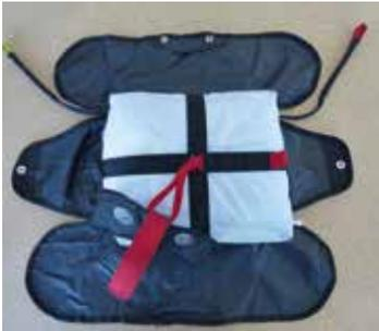
After that, lay the rescue parachute on top of the V-bridle lines in the middle of the front container.
