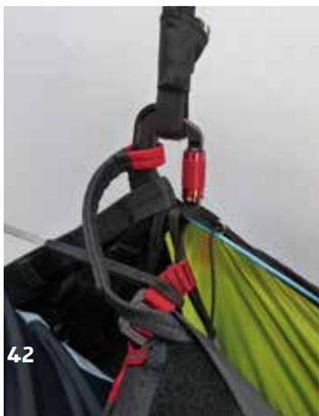
To ensure that the rescue handle is easily reachable and still deployable in the event of a line twist, make sure that the speedbag closing system passes through both loops on the outside of the front container.
