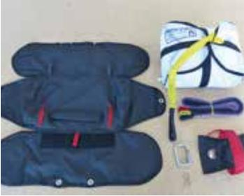
The reserve parachute consists of the parachute itself, the red rescue handle, the V-shaped bridle and the front container. The rescue handle on the front container is part of the RANGE AIR harness. This is the only rescue handle that may be used.
