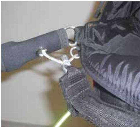
The function of the coupling and the rescue installation should be verified by a test release.
