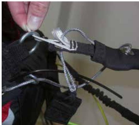
**3** After the gray line from the Separable Speed System is mounted correctly, pull the longer, white loop of the Leg Stirrups through the metal ring on the leading edge of the harness.
