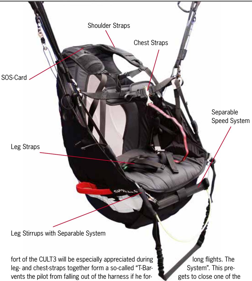
front of the CULT3 will be especially appreciated during long flights. The leg- and chest-straps together form a so-called “T-Bar” which prevents the pilot from falling out of the harness if he forgets to close one of the leg straps. The rescue handle, placed under the seat board (the handle is located on the right side) offers the advantage of providing clear sightlines forward and downward, and offers additional protection during a hard landing.
