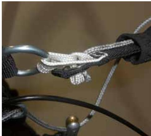
**4** The shorter, white loop should now be fed through the longer, white loop from above to below and then fed through the grommet of the leg stirrups. Here again, a support line can help with this procedure.
