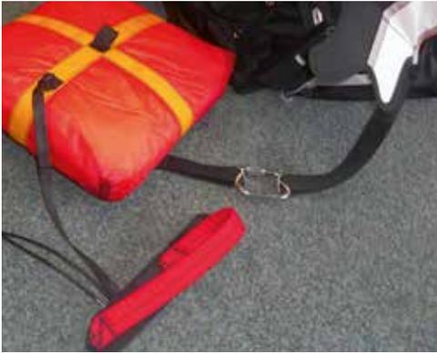
The CULT3 can be combined with most of the rescues currently on the market. The initial installation of the rescue must be tested by a certified compatibility controller. This procedure tests the functionality of the rescue activation and certifies the compatibility according to the rescue testing and packing documentation.
