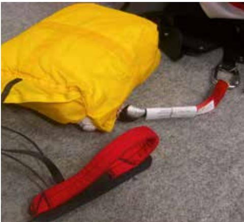
The permanent attached rescue handle and the inner container form a unit. This unit is packed in the outer container analog the above description.
