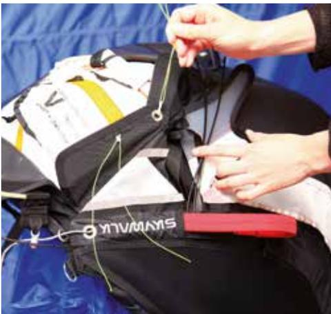
**3** After the rescue handle is secured on the harness, the outer container must be closed.
