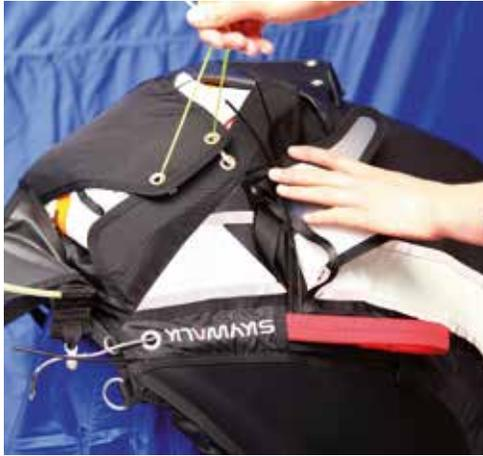
**4** Once the first grommet is fed through, feed on both grommets from the opposite sleeve.
