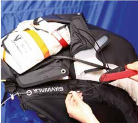
**1** The rescue is positioned in the outer container so that the connection lines and the rescue handle of the rescue are positioned on the right side of the harness. This way, the path of connection line and the rescue handle to the harness is direct and cannot become obstructed.
