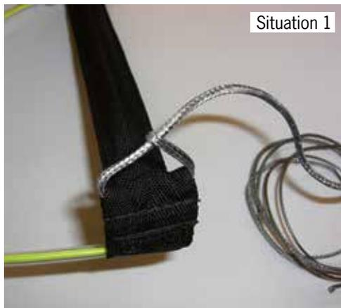
On the in-flight direction left side, the accelerator, as well as the Leg Stirrups is installed in the same manner as with most harnesses:
